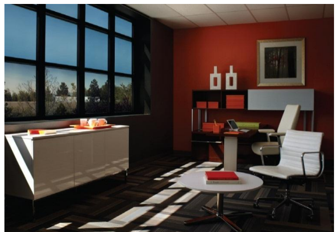
Figure 3.2 Image illustrating EC windows preserving view to outside while modulating solar transmittance. However, direct sun patches can be clearly seen even in the colored phase. (Source: Solardigm).
