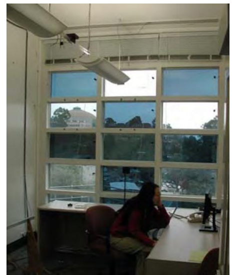
Figure 3.6 Photograph showing multiple EC windows installed side by side, resulting in checkerboard pattern. (Source: LNBL)
